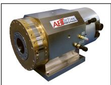
10,000 RPM SP138 with Foot mount housing, liquid cooled, brushless DC motor and optical encoder for work holding or grinding applications.
