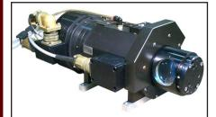
20,000 RPM air bearing spindle for 3-Dimensional imaging system. Brushless DC motor drive and optical encoder with capacitance probe gap monitoring system.
