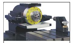
10,000 RPM Air bearing spindle with custom chuck, A-thermal mount housing, brushless dc motor and optical encoder for diamond turning of high precision valve bodies.
