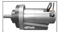
3,000 RPM air bearing spindle. SP38 Compact design constructed of hardcoated aluminum with brushless dc motor drive, optical encoder and vacuum feed through the center for work holding.
