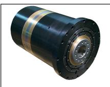
5,000 RPM SP180 air bearing spindle for work holding applications. Integral brushless dc motor and optical encoder with vacuum feed thru center.
