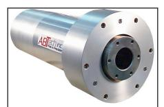
20,000 RPM air bearing spindle for diamond turning of contact lenses. Integral Brushless DC motor and optical encoder, dual plane balanced and liquid cooled housing.
