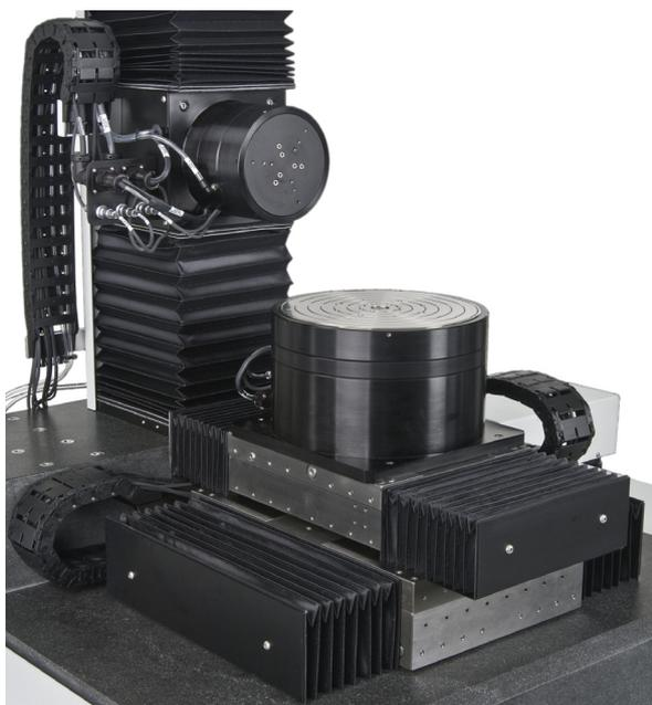
ABTech 5 axis air bearing optical metrology platform
